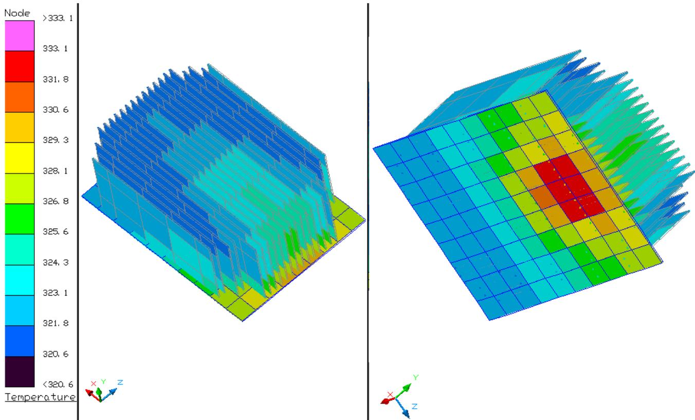
**Figure 4: Automatically Optimized Heat Sink (Cover Removed)**
