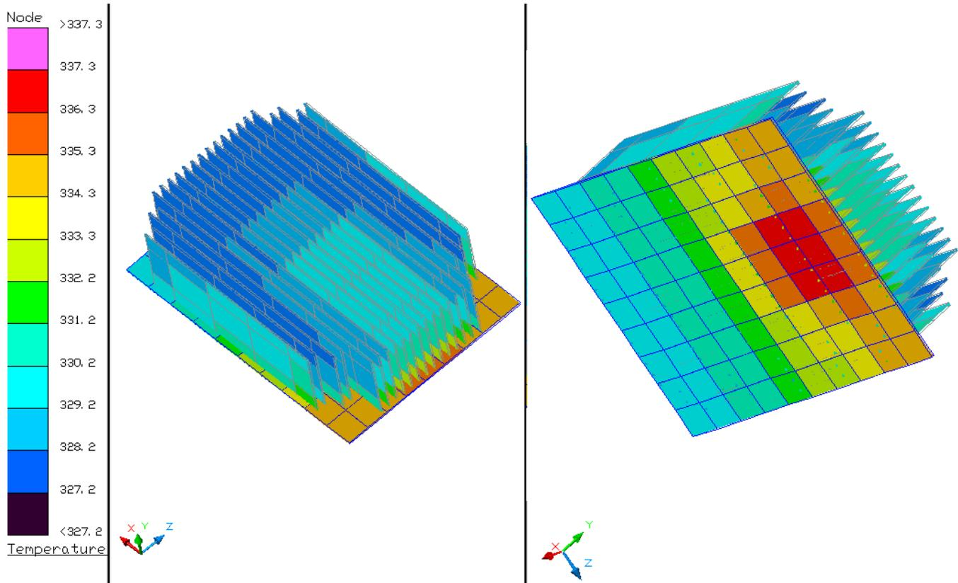
**Figure 3: Initial Configuration/Performance of Heat Sink (Cover Removed)**
