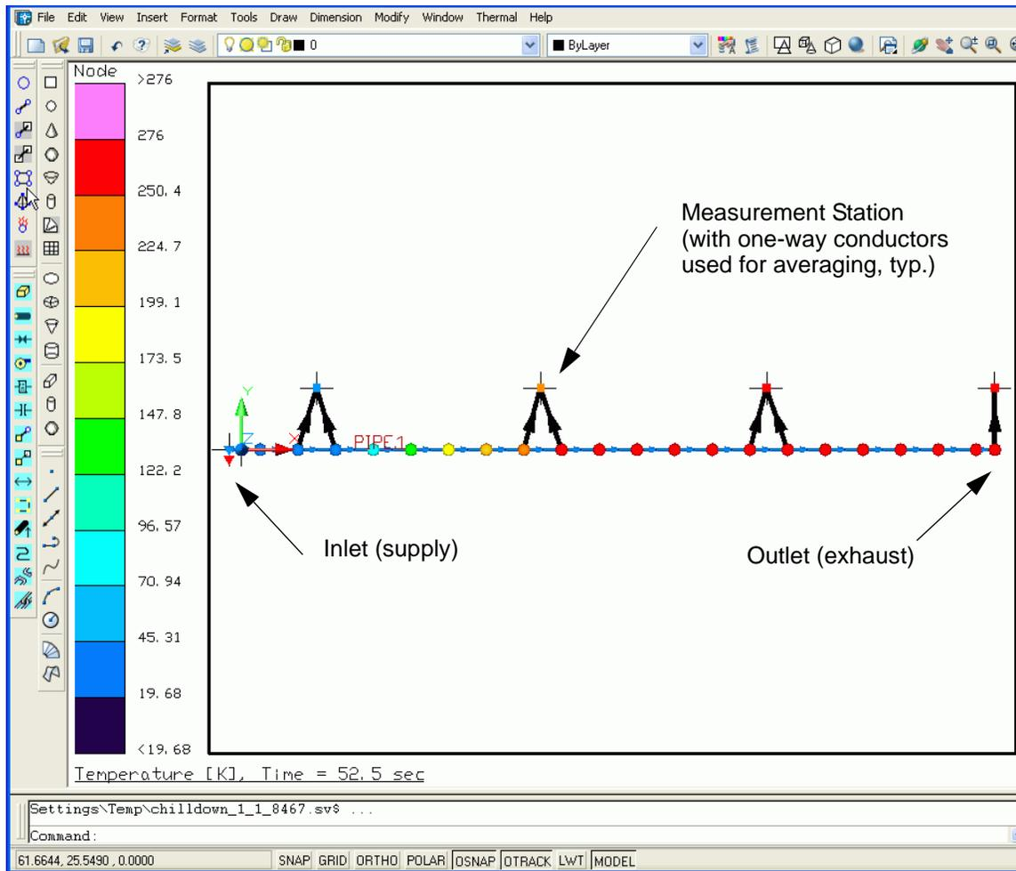
Figure V-2: Thermal Desktop Depiction (postprocessed in middle of run) of Model
