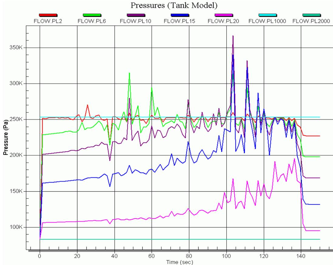
Figure V-6: Pressure Histories with Full Hydrodynamics (Tanks instead of Junctions)
