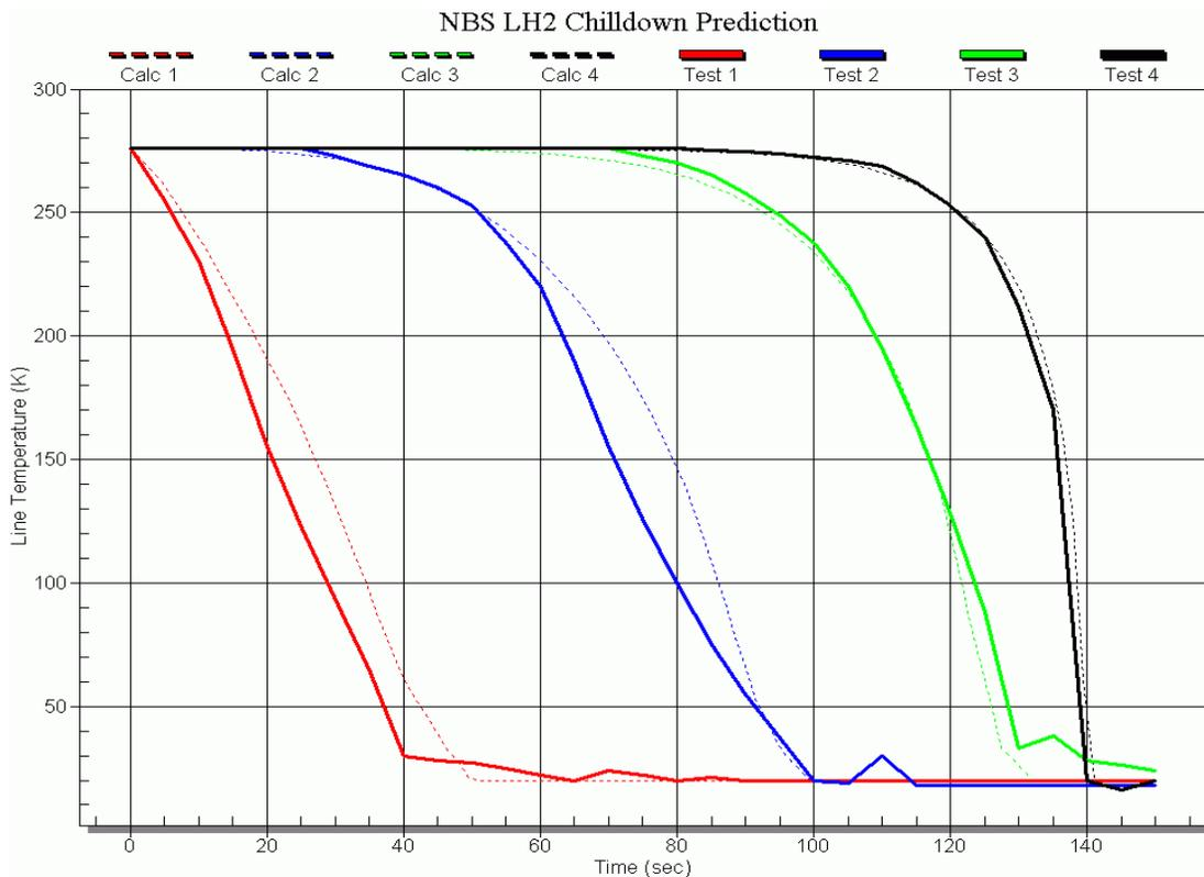
Figure V-4: Comparisons of SINDA/FLUINT Predictions with Test Data
